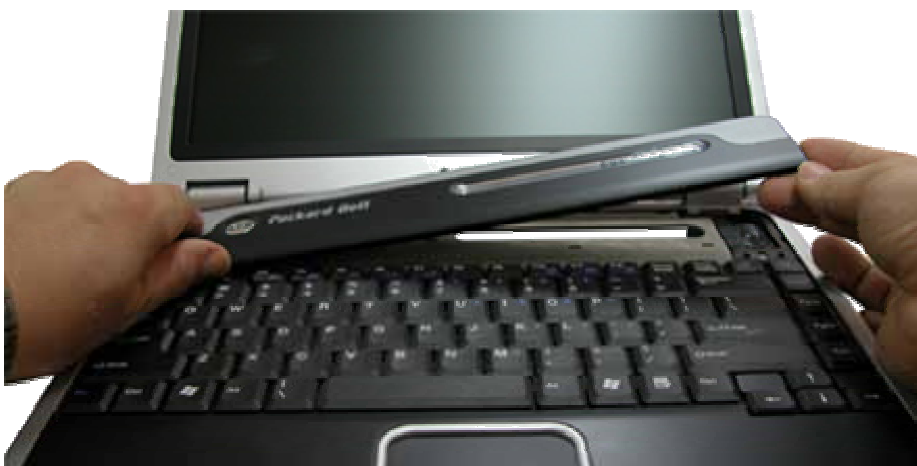
Fig. 15 Lifting up Keyboard Cover
